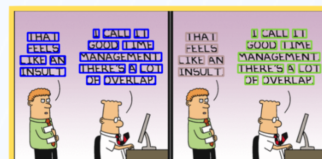
Fig 4. Example of bounding box clustering. The original bounding boxes (left) and the identified clusters (right)
