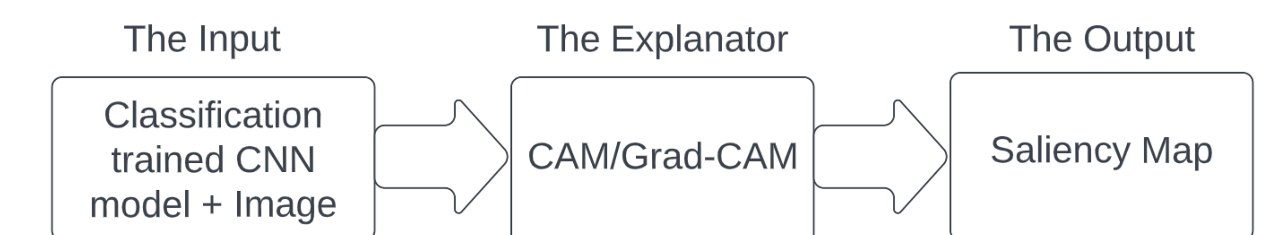
Figure 2: The building blocks of an XAI system following the CAM and Grad-CAM techniques.
