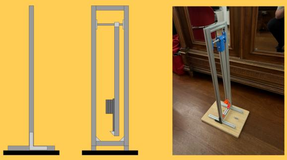
Made from 20mm aluminum extrusions and 3D-printed mounting brackets. IMU chips of devices aligned by overlaying motherboard schematics and placing the Midge on the correct place of the phone.
