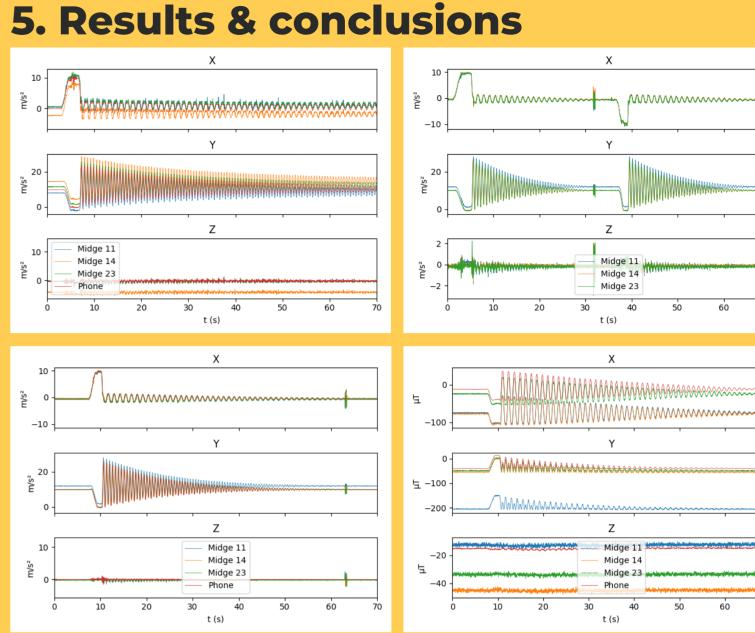
Data timing was manually aligned by looking at the graphs and offsetting the data. This was required since the timestamp were not syncronized exactly and the phone used another timestamping system and had a 100Hz sampling rate instead of approximately 57Hz for the Midges.
