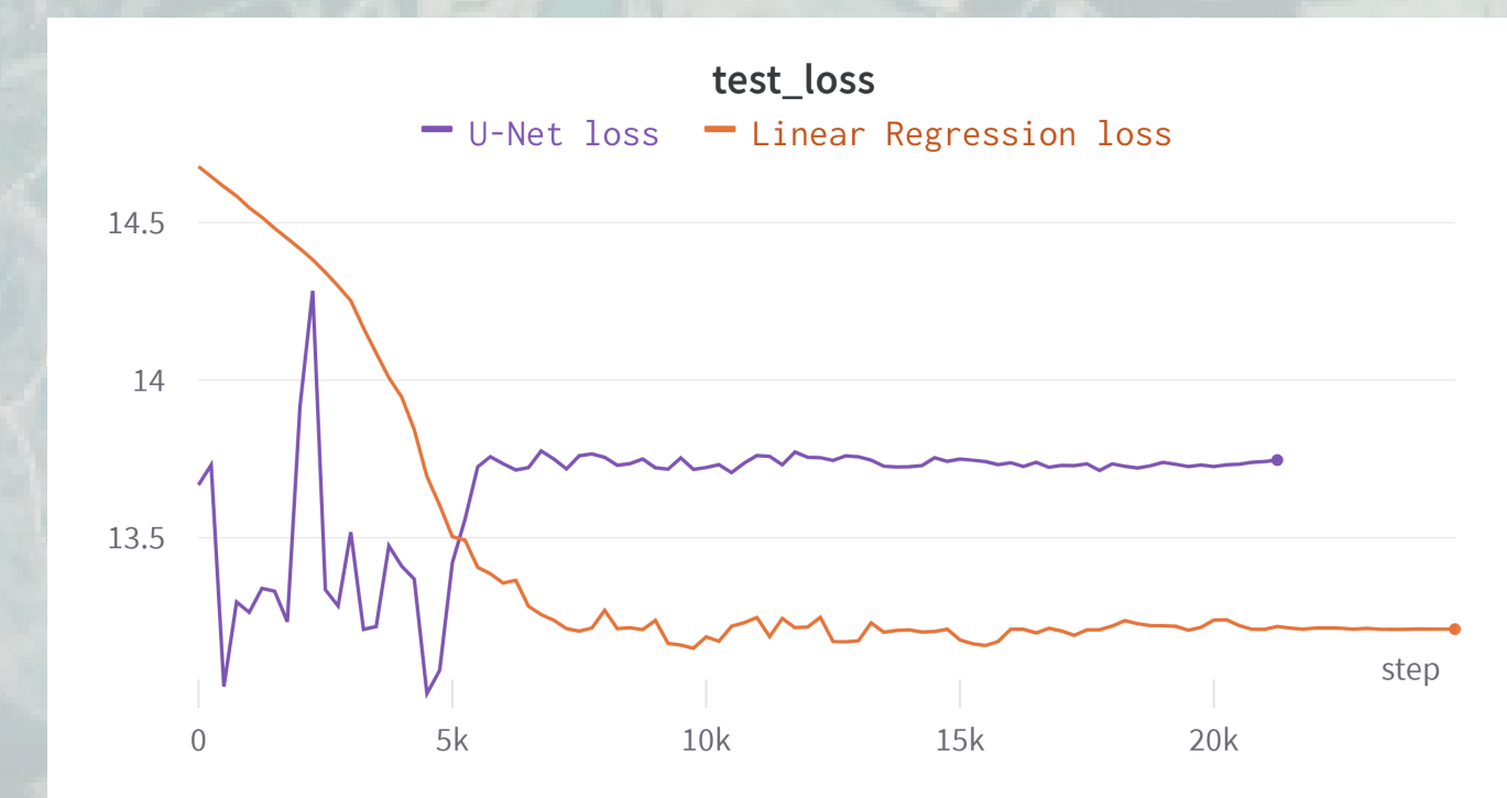
Fig. 1 U-Net / Linear Regression losses. x-axis: epochs, y-axis: loss. Every 250 samples the models are evaluated against test set
