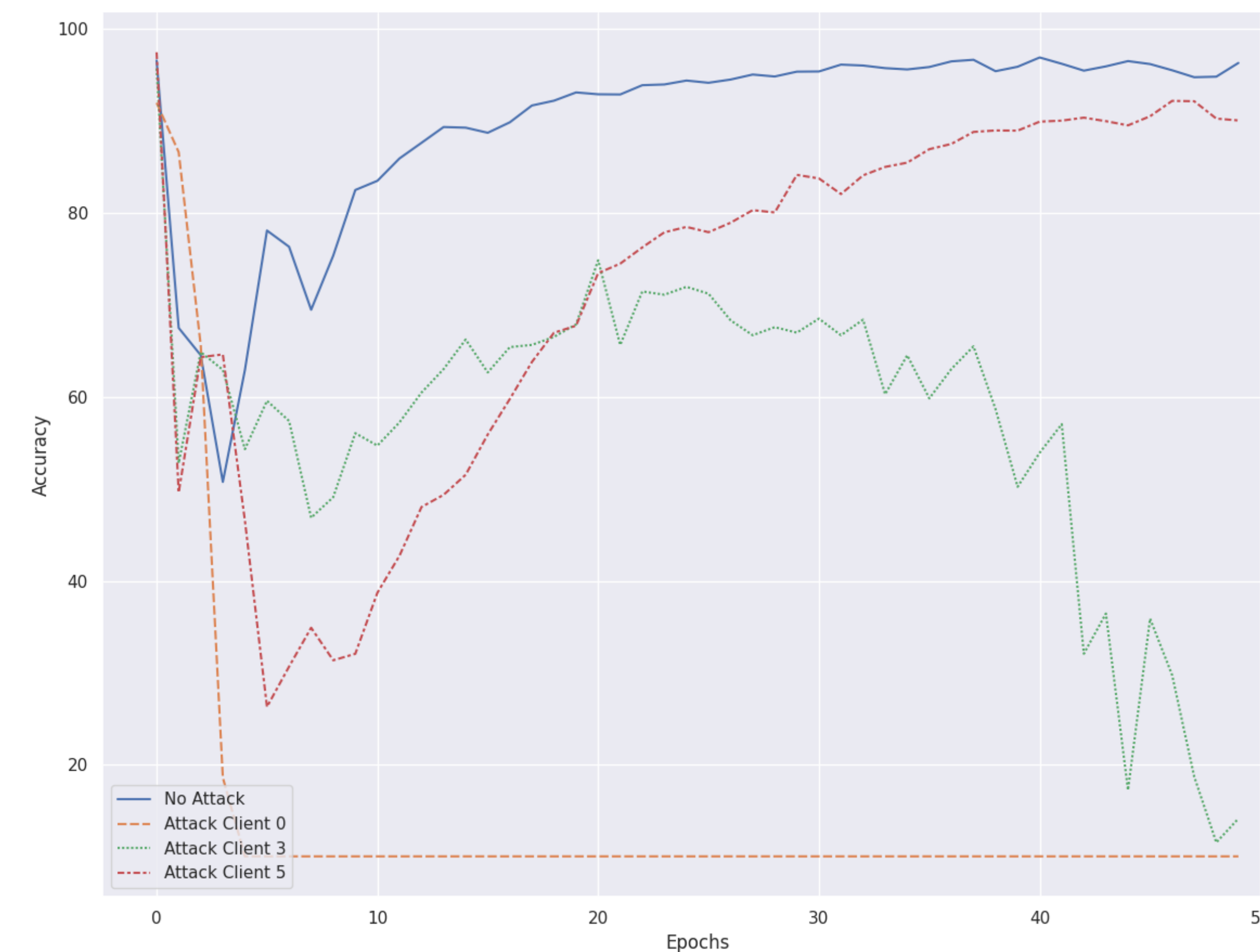
Figure 2: Comparison of the effects of an multi-server adaptation of the single-server attack MinMax[2] carried on a network from differently located malicious client. The malicious client in an overlapped region is able to be very effective, while those within a reach of a single server can barely affect the accuracy.
