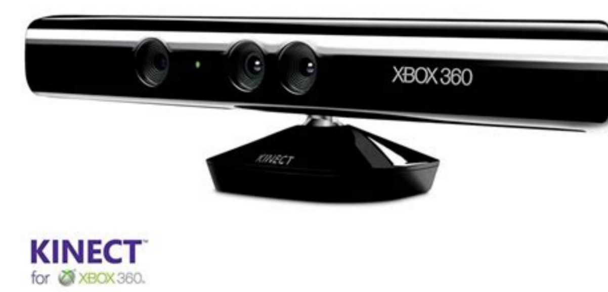
Figure 1. The Microsoft Kinect, a camera-based sensor used for HPE
