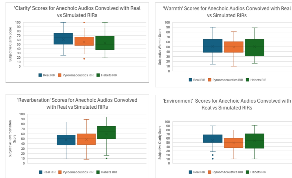
Results per attribute for the modified Multiple Stimuli with Hidden Reference and Anchor (MUSHRA) test (0-100)
