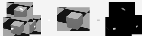
Fig. 4. The calibration step for 3 of the projector's pixels. For every pixel in the projector, a picture is taken. The picture where all projector pixels are off is subtracted from these pictures. The results are stored in the calibration matrix.
