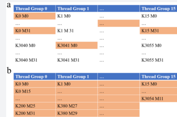
Figure 3: Thread group level load balancing [2]
