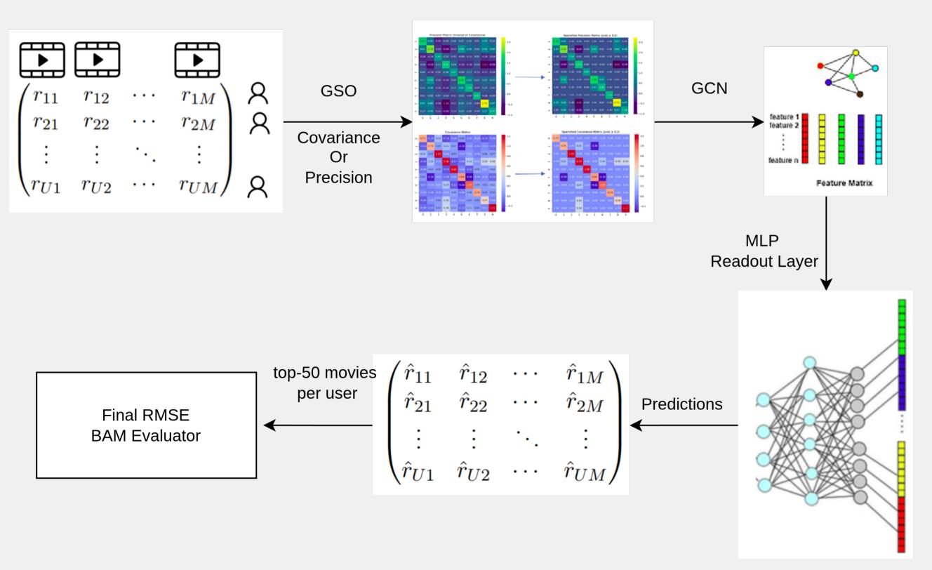
Outline of the model: Data  $\rightarrow$  Graph Shift Operator (Cov/Prec, sparse/dense)  $\rightarrow$ **SelectionGNN** filter bank  $(K=2) \rightarrow$  read-out  $\rightarrow$  Top-50 ranking  $\rightarrow$  BAM evaluation.
