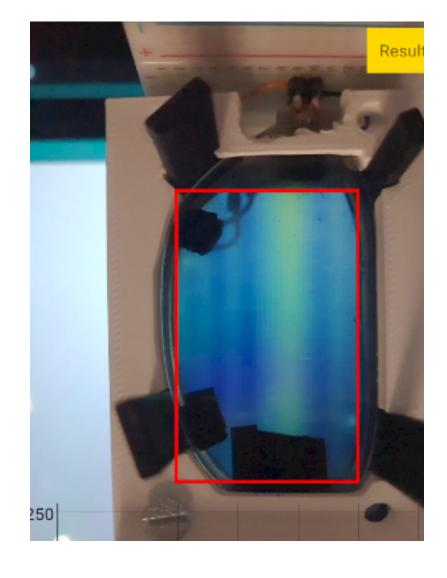
With the location of the transmitter known, the red green and blue values of the columns can be summed up, and the data can be decoded.
