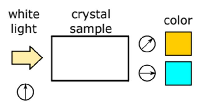
By applying a voltage over a liquid crystal cell, the color can be changed. Depending on the voltage different colors are produced.
